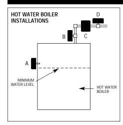
HOT WATER BOILERS: Probe must be installed at or above the minimum safe water level established by the boiler manufacturer. The probe may be installed directly in the boiler if a suitable tapping is available (A), in the riser (B), or in the header (C) or (D).
