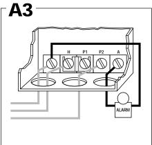
■A3 Optional alarm connection. Connect alarm common to terminal GN. Connect alarm hot to terminal A.
