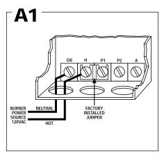
VAT Connect the hot lead of the input voltage (120 VAC, 60 HZ) to terminal H. Connect the neutral lead to terminal GN. 120 VAC, 60 HZ must be supplied to terminals H and GN for internal operation of the control.
