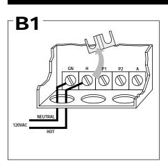
■ ■ WARNING! Remove the jumper between H and P1. Connect the hot lead of the input voltage (120 VAC, 60 HZ) to terminal H. Connect the neutral lead to terminal GN. 120 VAC, 60 HZ must be supplied to terminals H and GN for internal operation of the control.
