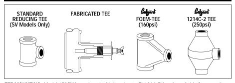
**TEE MOUNTING:** Model 170**SV** is equipped with the shorter EL1214-SV probe suitable for mounting in standard reducing tees. For other 170 Series controls, a fabricated tee can be used. Make sure that the tee drains thoroughly when water falls below it and that it conforms to the spacing requirements described in Step 3. Safgard tees are also available to accommodate all probe models (See page 4).
