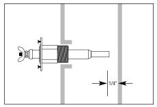
Check to insure 1/4" clearance from the probe to any surface within the boiler or tee. Apply pipe sealing compound to threads.
