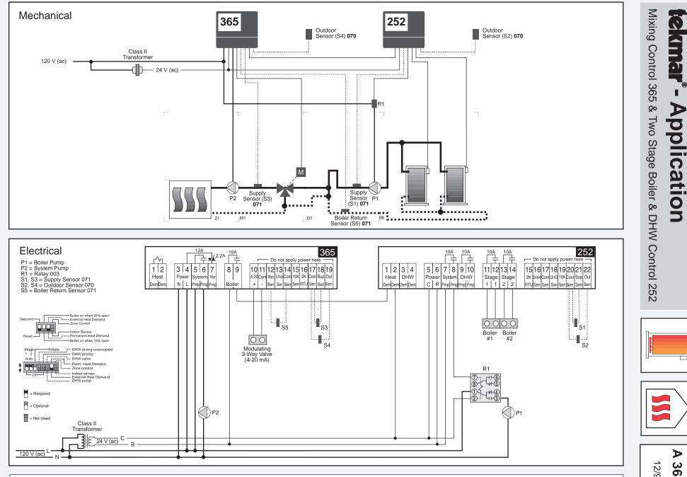
Note: This is only a concept drawing. The designer must determine whether this application will work in his system and must ensure compliance with code requirements. Necessary auxiliary equipment, isolation relays (for loads greater than the specified tekmar internal relay ratings), and other safety and limit devices must be added.
