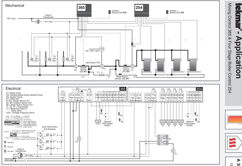
Note: This is only a concept drawing. The designer must determine whether this application will work in his system and must ensure compliance with code requirements. Necessary auxiliary equipment, isolation relays (for loads greater than the specified tekmar internal relay ratings), and other safety and limit devices must be added.
