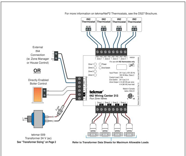
**Description:** tN2 Wiring Center 313, four tekmarNet®2 Thermostats, and four zone valves wired into a powered boiler demand input on a device such as a tekmar Boiler Control 260.
