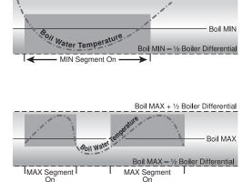
Boil MIN + 1/2 Boiler Differential
