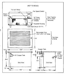
Heat Exchanger. Highly efficient dual circuited headered coil, made of copper alloy tubes brazed with lead free solder and expanded into smooth aluminum plate fins (10FPI), tested to 300psi, and sealed for quality. It's positioned in the unit for maximum heat transfer across the coil.
