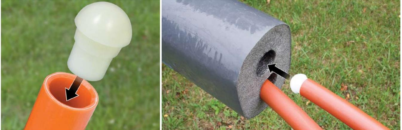
Guide and slide the first length of pipe all the way through to the opposite end of the MAXX-R insulation. Slide the second length of pipe through the second opening in the MAXX-R insulation until it passes through to the end of the first 8 foot piece of insulation.
