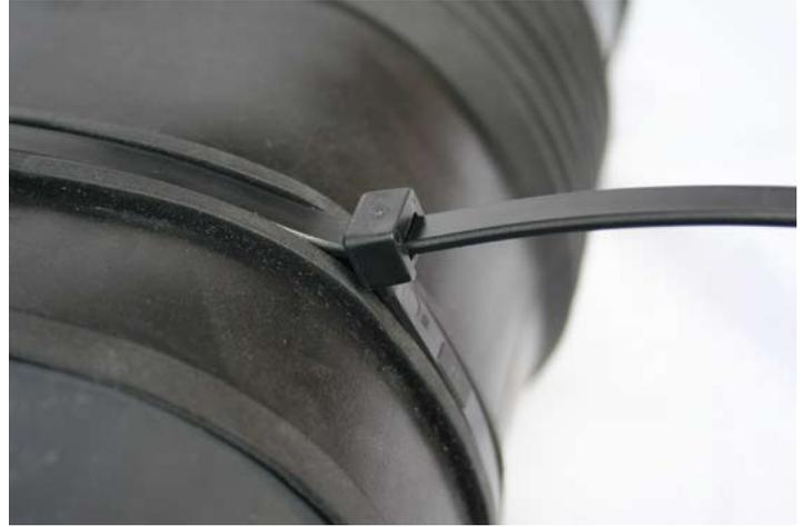
Once completed, take the two high density cable ties provided and place on each end of the boot. (You will note there is an indentation guide showing the location for the ties on each end). Once the ties are in place, pull (or secure) each tie to secure the boot onto the MAXX-R. Do not over tighten. 1/16” to 1/4” indentation is adequate; however, an indentation is necessary.
